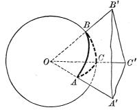
triedral angle will be three arcs of great circles of the sphere, forming a spherical triangle, as ABC. The sides (arcs) AB, BC, CA of this triangle measure the face angles A'OB', B'OC', C'OA' of the triedral angle. The angles ABC, BCA, CAB, are measured by the plane angles which also measure the diedral angles of the triedral angle; for, by Geometry, each is measured by the angle between two straight lines drawn, one in each face, perpendicular to the edge at the same point.
