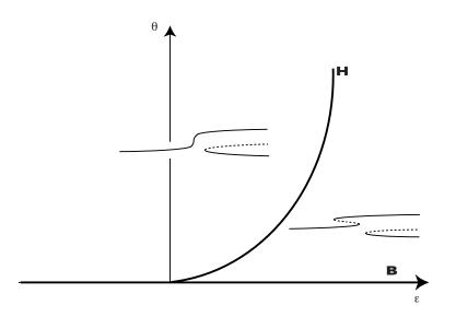
Figure 1: Bifurcation and hysteresis sets (in bold) in the positive half-plane. The bifurcation diagrams drawn (on the  $(\mu, p)$ -plane) remain qualitatively equivalent in each connected component. A solid line in a bifurcation diagram represents stability while a dotted line means the branch consists of unstable equilibria.
