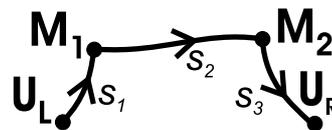
FIGURE 5.4. Local solution for saddle equilibrium. Waves: 1-shock ( $U_L, M_1, s_1$ ); transitional ( $M_1, M_2, s_2$ ); 2-shock ( $M_2, U_R, s_3$ ).
