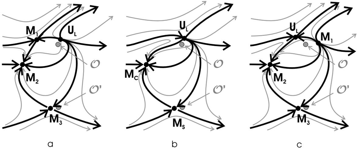
FIGURE 4.10. Phase portraits for  $U_L \in T(\beta)$  with different speeds: a)  $s \lesssim s_0$ ; b)  $s = s_0$  (the equilibrium  $M_1 = U_L$  is a repeller-saddle); c)  $s \gtrsim s_0$ .
